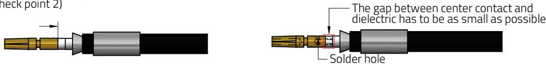
**Step 4.** Push cable with center contact into connector main body until perceptible point. Cover cable braid over connector neck carefully
